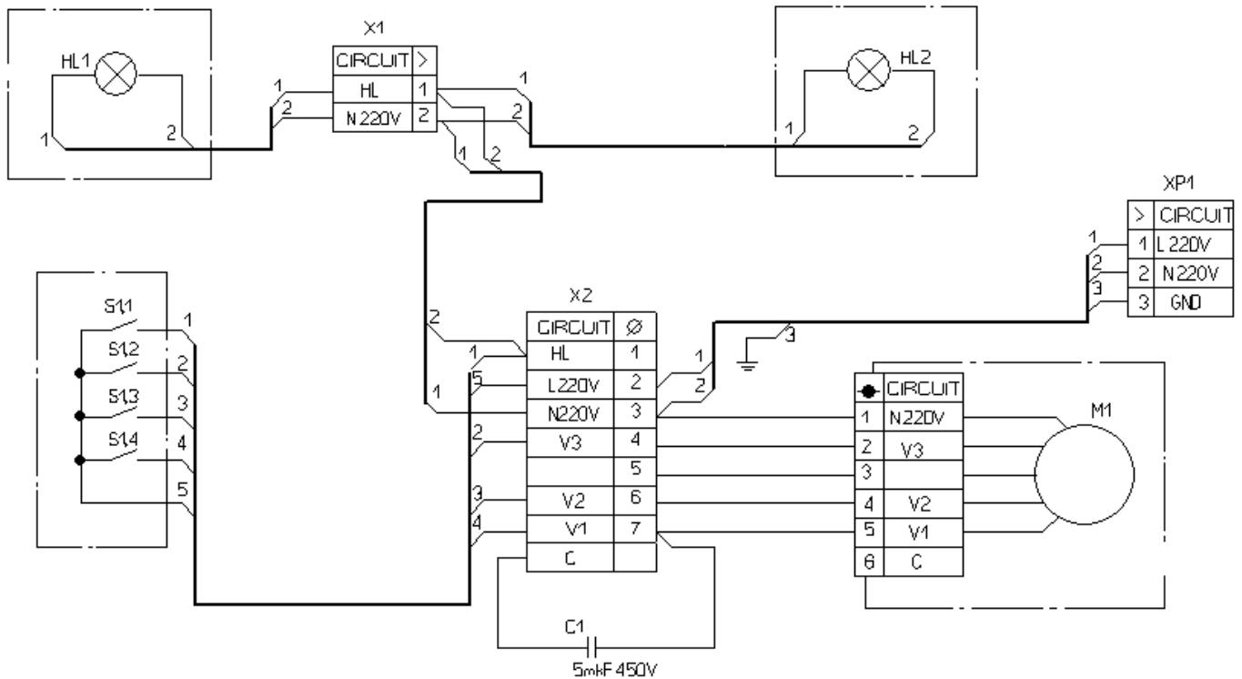
**Electrical schematic diagram of the sensor extractor hood «HIT PLUS» with capacity (520/700 mm)**
